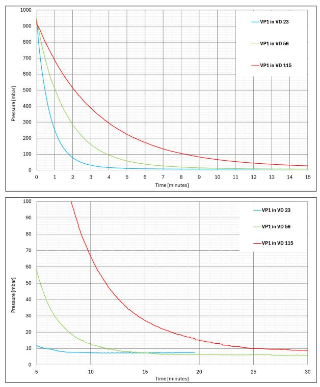
Pump-Down Charts of VP1 with Vacuum Ovens of Series VD
